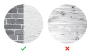
Grab 4 of the wall anchors from Bag A. Using your Ring Doorbell as a template, mark 4 drill holes on the wall. Use a 6mm masonry drill bit (not included) to drill the holes, then insert the
